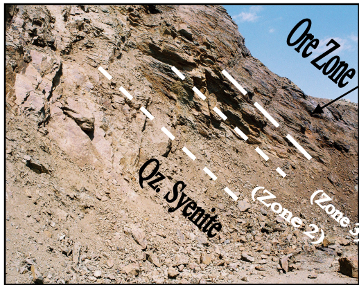
Fig.7 -Ore body and its spatial relation with quartz syenite footwall in the Baba Ali deposit.
